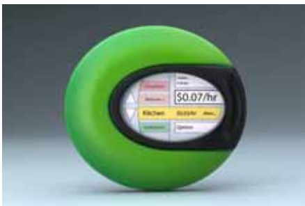
Runner-up: wireless electricity metering system
